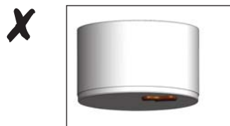
Figure 15 Excessive food spillage stuck to pan base will impinge balance of pan. One side of utensil will be further away from induction field than another. This may reduce efficiency and will cook one side of pan faster. Keep pans clean to ensure efficient cooking.
