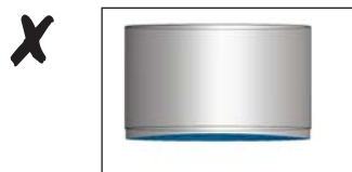
Figure 14 Pot base is bowed inward and is NOT FLAT; The unit efficiency will be dramatically reduced during cooking. It may not even be detected.
